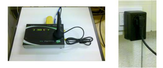
Figure 3.6: Digi Connectport X4 gateway and smart plugs.
