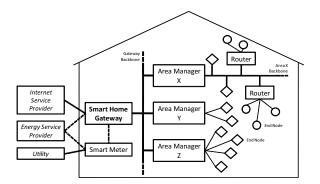
Figure 2.2: The Smart Home network architecture.
