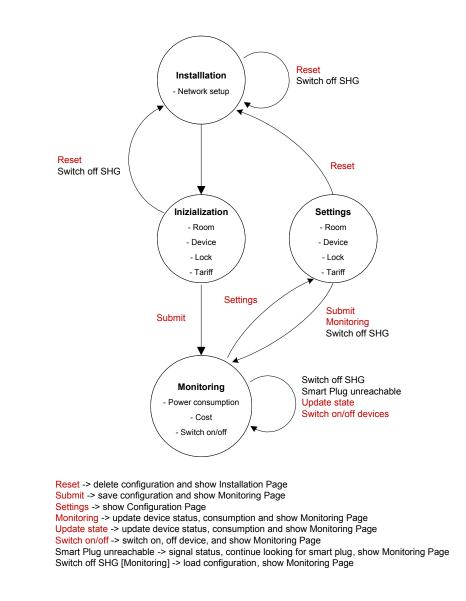
Figure 3.2: State diagram of the EMS. Red text indicates commands, while black unexpected situations.
