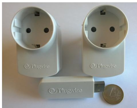
Figure 2.2: Plugwise kit for HEMSs: smart plugs and stick USB-Zigbee.
