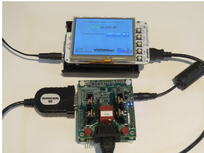
Figure 5.4: The embedded PC and the PLC interface of the SHG on top and bottom, respectively.
